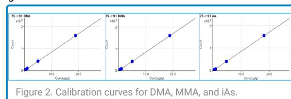
Figure 2. Calibration curves for DMA, MMA, and iAs.
