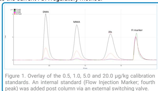
Figure 1. Overlay of the 0.5, 1.0, 5.0 and 20.0 μg/kg calibration standards. An internal standard (Flow Injection Marker; fourth peak) was added post column via an external switching valve.
