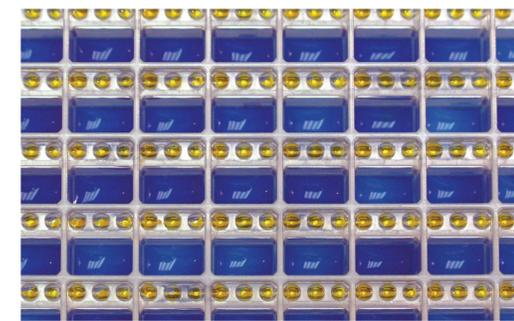
**Figure 5:** Actual photo of a Greiner 963 Crystallization plate with each main reservoir containing 80 μl of blue dye solution and three different drop volumes of 10% Tartrazine dye solution on the three top shelves. The drop volume in each top shelf is 300 nl, 200 nl and 100 nl respectively. Drops were dispensed with the Honeybee 963 System.
