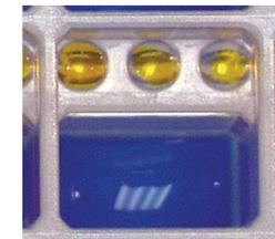
**Figure 4:** Enlarged image of a single well on a Greiner 963 Crystallization plate with three drops of 10% Tartrazine dye solution. Drop volumes are 300 nl, 200 nl and 100 nl respectively.
