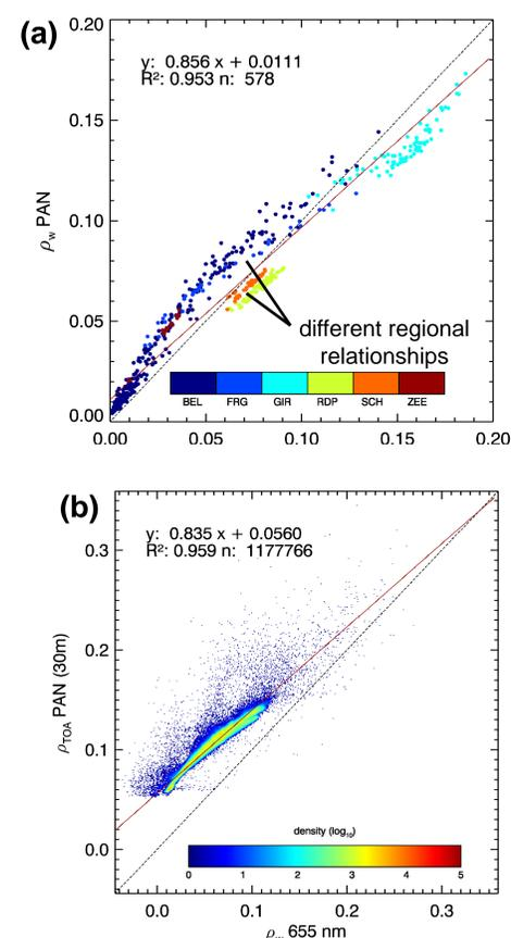
Figure 2 Scatter plots showing the relationships between reflectances in the panchromatic and red channels of OLI, (a) derived from in situ TRIOS hyperspectral measurements of  $\rho_w$ , (b) scatterplot of  $\rho_{TOA}$  PAN (resampled to 30 m) and  $\rho_{TOA}$  655 nm. Dashed lines are the 1:1, the solid red lines are the OLS linear regression lines. Colours denote (a) sampling region and (b) pixel density.
