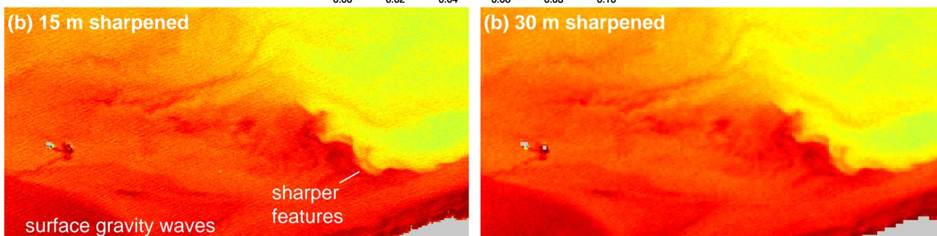
Figure 3  $\rho_w$  655 nm derived from a subset of Landsat-8/OLI scene LC81990242014075LGN00 using [VR2015] (a) at 30 m native resolution (b) after sharpening using the 15 m panchromatic band. At 15 m, spatial features are sharper, and surface gravity waves are in many cases spatially resolved.
