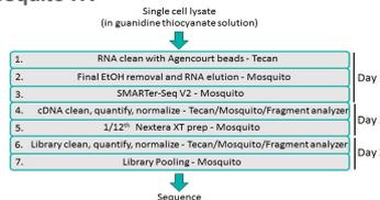
Fig. 5 Low-volume SMART-Seq2 workflow at the MIT BioMicro Center
