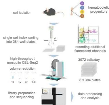
Fig. 2 Miniaturized cDNA synthesis protocol for 384-well scRNA-seq using the mosquito LV, modified from Hashimshony *et al.* (3).
