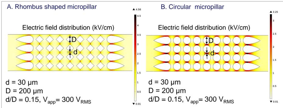
Comparison of distribution of electric field (kV/cm) for two microfluidic devices with; (A) rhombus shaped micropillar and (B) circular micropillar. Darker region indicates higher magnitude of electric field.
