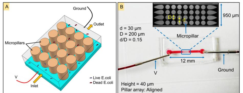
Above figures depicts (A) schematic of our microfluidic device and (B) PDMS-glass microfluidic device. Microchannel was fabricated using standard soft lithography technique.
