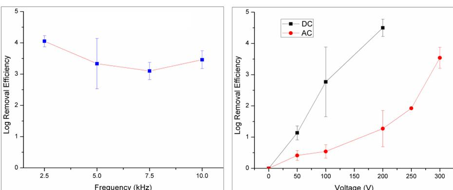
Figure (A) shows the effect of applied AC frequency on log removal efficiency of *E. coli* under an applied AC voltage of 300 V and flow rate being 1 mL/hr.
