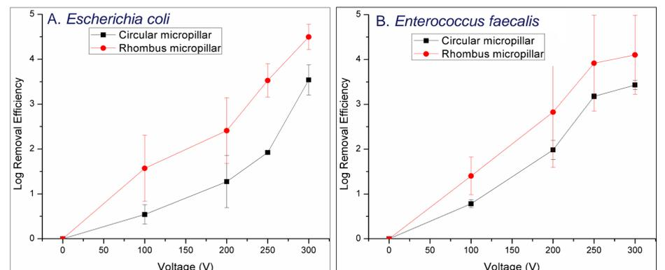
(A) Comparison of log removal efficiencies for *E. coli* (gram-negative bacteria) for microfluidic devices with rhombus shaped micropillars and circular micropillars
