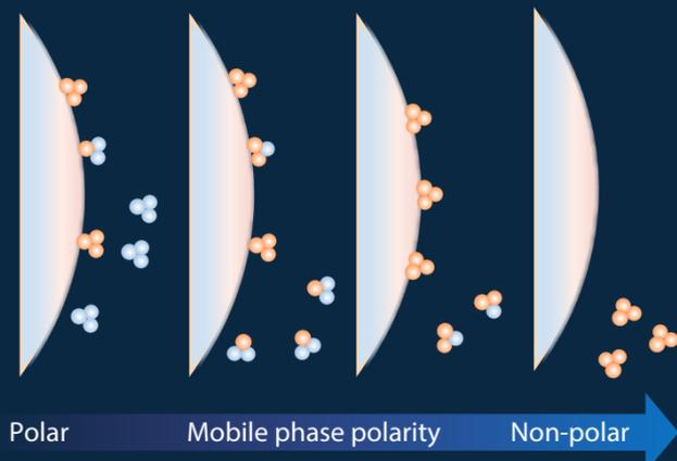
Most commonly used HPLC type with a non-polar stationary phase and an aqueous, polar mobile phase. Separations based on an analytes relative affinity for the mobile phase versus the stationary phase. In RP-HPLC, hydrophobic molecules tend to interact with the stationary phase, whereas hydrophilic molecules elute first.
