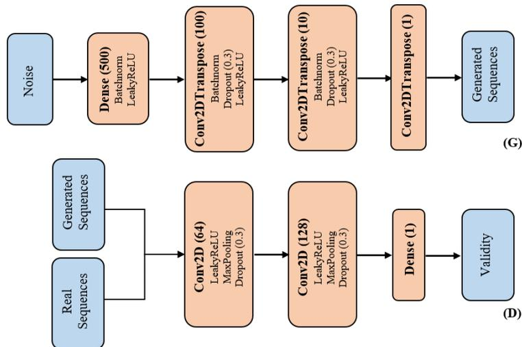
Figure 1. The architectures of Generator (G) and Discriminator (D) models.
