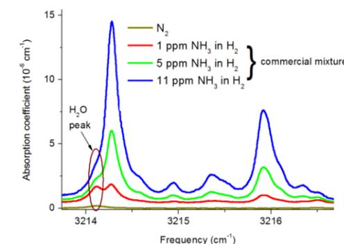
**Figure 4** Measurement of 3 ammonia in hydrogen mixtures
