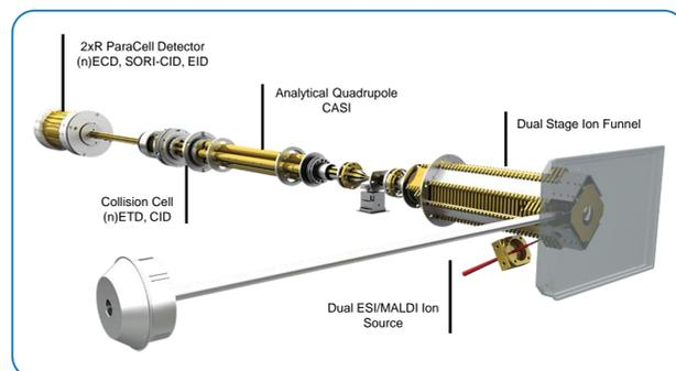
**Figure 2:** Schematic of the ion path of the scimaX<sup>®</sup> MRMS system used for the analysis of fragile protein-drug complexes under native conditions.
