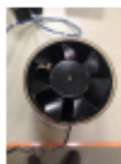
This is the circulator used in this experiment. It is a six inch direct current tubaxial fan (Ebm-papst, Inc., Farmington, CT) that is mounted inside of a carbon dioxide absorber with no soda lime. This circulator was powered by a Tektronix power supply.
