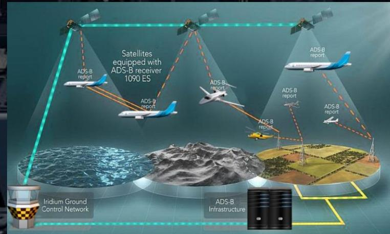
**ADS-B In** provides operators of properly equipped aircraft with weather and traffic position information delivered directly to the cockpit. ADS-B In-equipped aircraft have access to the graphical weather displays in the cockpit as well as text-based advisories, including Notices to Airmen and significant weather activity.
