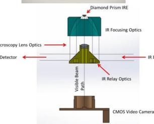
Optical Diagram (bottom) and photograph (top) of MicromATR™ Vision
