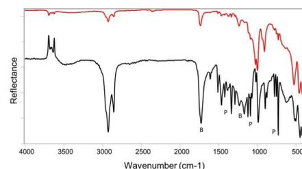
**Right, top** – unprinted, coated paperboard. Dominated by the pigment in the coating, kaolin and the binder. A triplet of  $\nu\text{OH}$  bands at 3690, 3650, and 3620  $\text{cm}^{-1}$  and strong Si-O and Al-O bands in the 1000-800  $\text{cm}^{-1}$  range are indicative of the kaolin. Bands at 1736 ( $\nu\text{C=O}$ ) and 1238  $\text{cm}^{-1}$  ( $\nu\text{C-O}$ ) are consistent with a polyester binder.
