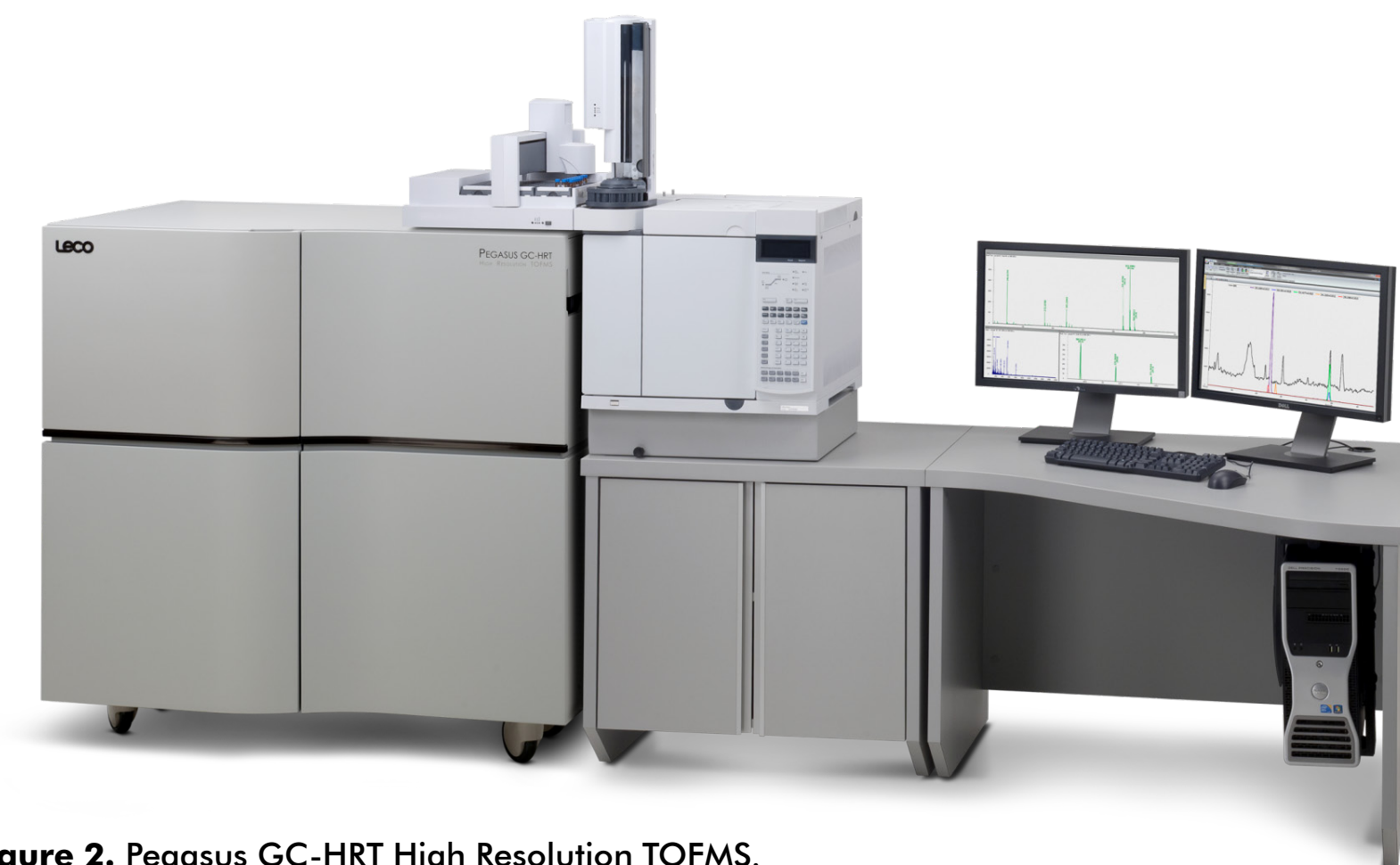
Figure 2. Pegasus GC-HRT High Resolution TOFMS.
