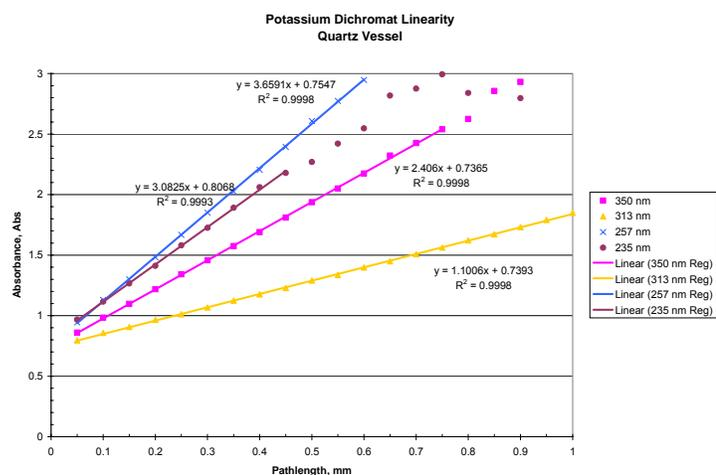
**Figure 5: Quartz Vessel Measurements**
