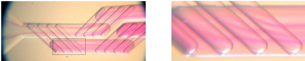
Left: Low magnification view of the junction. Right: Magnified view of the region marked in the left image. Streaks are visible as having doubled in number from 2 to 4. 4 streaks are visible towards the right end of the image.
