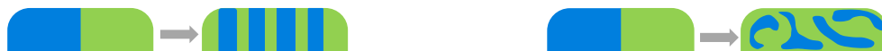
An inlet feed of two adjacent concentrations enters. Left: Laminar flow and diffusive mixing – At low flow rates, the flow is split horizontally into 4 lamellae. The split streams are re-joined side by side. The widths of the lamellae decrease as they reshape to the minimum channel cross section. Right: Chaotic flow and advective mixing – at higher flow rates, swirling and turning of the flows result in marble-like mixing.
