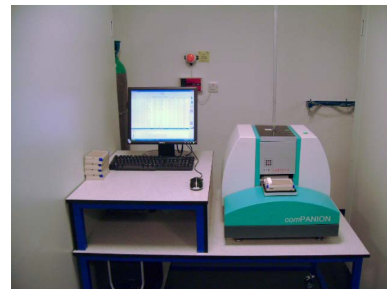
Figure 3. TTP Labtech's comPANION linked to and controlling throughput of 2 neighbouring comPOUND modules
