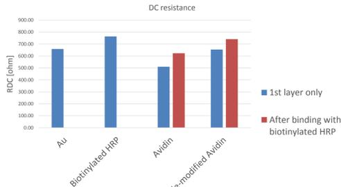
Fig. 3: DC resistances of the voltammograms in figure 2
