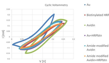
Fig. 2: Voltammograms of different protein formations and bare gold
