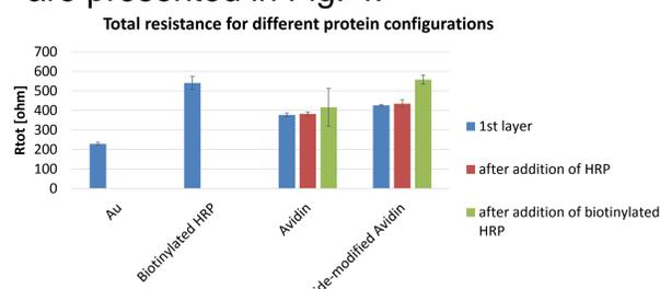
Fig. 4: Total resistance ( $R_e + R_{e,p} + R_{ct}$ ) calculated for different protein configurations
