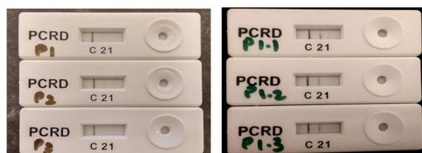
Direct detection on a NALF device of a negative control.
