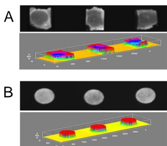
Chitosan functionalised regions of A) pipette deposited patterning of paper strips and B) Dip-coated paper reaction discs and the corresponding three dimensional topography of the chitosan modified regions.
