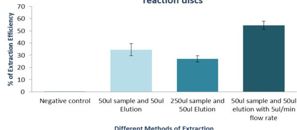
Adjusting the flowrate increased the extraction efficiency to 57%. This can be considerably increased by fine tuning the parameters.
