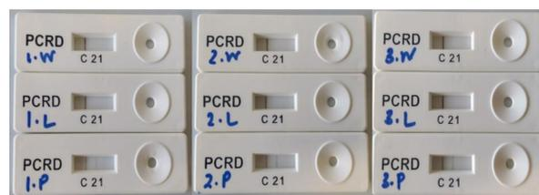
RPA of CT gDNA on paper with end-point detection on NALF devices. The plastic support that held the membranes were also washed with the LF running buffer and tested to determine amplification only proceeded within paper matrices
