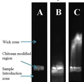
DNA extraction on a chitosan functionalised  $\mu$ PAD (paper strip). A) Negative control B) FAM tagged DNA sample (pH 5.0) captured onto the chitosan modified region C) Elution of DNA sample with the introduction of pH 9.0 Tris/KCl buffer.
