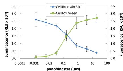
HCT116 cells were cultured in InSphero GravityPLUS<sup>™</sup> 3D Cell Culture system for 4 days to form ~350 μm microtissues. Samples were treated with CellTox<sup>™</sup> Green and panobinostat for 48 hr. After recording fluorescence, an equal volume of CellTiter-Glo<sup>®</sup> 3D Reagent was added, the plate was shaken for 5', and the luminescence was recorded after a 30' incubation.
