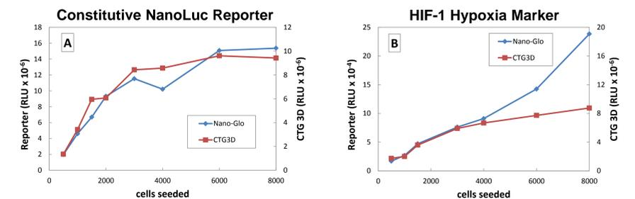
HCT116 cells expressing NanoLuc luciferase under a constitutive promoter (A) or a HIF-1 promoter (B) were cultured in InSphero GravityPLUS<sup>™</sup> 3D Cell Culture system for 4 days to form ~200-700 μm microtissues. An equal volume of NanoGlo Reagent or CellTiter-Glo<sup>®</sup> 3D Reagent was added to each well, the plate shaken for 10', and luminescence recorded after a total of 30 min incubation.
