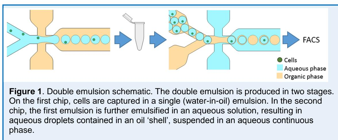
FACS, and the 30  $\mu\text{m}$  droplets are small enough to pass undamaged through the sorting cell. Here, we investigate the use of a two-chip system for making 30  $\mu\text{m}$  double emulsion droplets.
