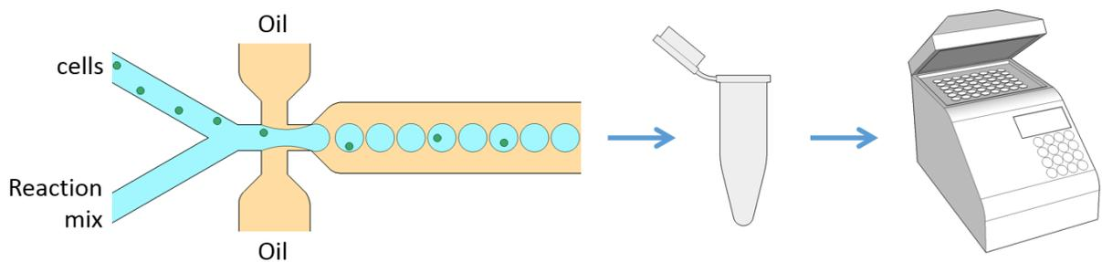
**Figure 1.** In a typical experiment, cells are combined with a reaction mix, such as an RT-PCR mix, and encapsulated in droplets in oil. The resulting micro-emulsion is collected, typically in a chilled PCR tube, and transferred to a PCR machine for RT-PCR.
