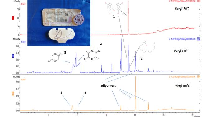
Figure 3: Coated Suture 150C (Top), 300C (Middle) & 700C (Bottom)
