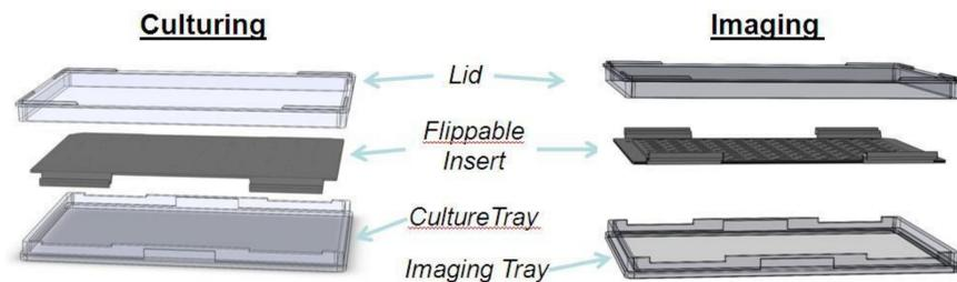
**Figure 1: Schematic of the  $\mu$ ALI Plate.** The  $\mu$ ALI Plate consists of a single 96-well flippable insert which allows liquid handling access and contains both the basal and apical sides of the device. The insert can be placed in a culturing tray for cell culture or removed and placed in an imaging tray for high content imaging.
