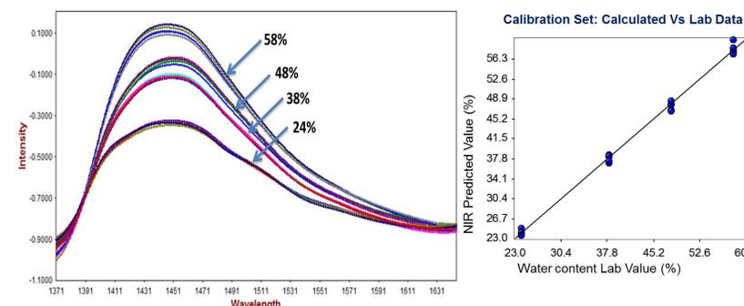
Fig.5: shows the water absorption region of the NIR absorption spectra of the contact lenses with various percentages of embedded water collected using RCA in trans-reflectance mode. The standard error of calibration using only two factors was 0.82 % with an R<sup>2</sup> value of 0.9964.
