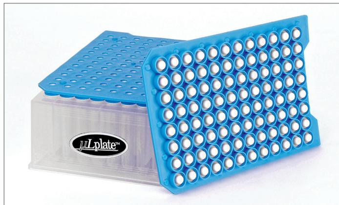
Figure 4 - CapMat with Sample Plate (with Inserts)
