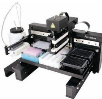
**Figure 2** – The Precision™ Microplate Pipetting System combines an 8-channel pipetting head and an 8-channel bulk reagent dispenser in one instrument. The instrument was used to dispense U937 cells, serially titrate antibody across a 96-well PP plate, transfer samples from plate to plate, as well as for TNF $\alpha$  and reagent dispensing.
