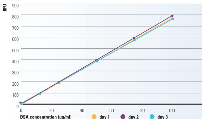
**Figure 2.** BSA standard curves prepared on three different days with a manual Finnpiquette using the forward pipetting technique
