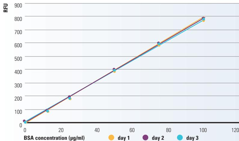
**Figure 1.** BSA standard curves prepared on three different days with a Finnpiquette Novus Electronic Pipette using the Dilute and Mix mode
