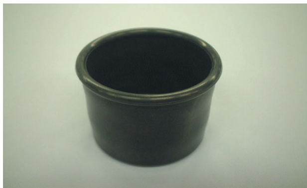
Fig.1 Black Rubber Diaphragm Test Sample
