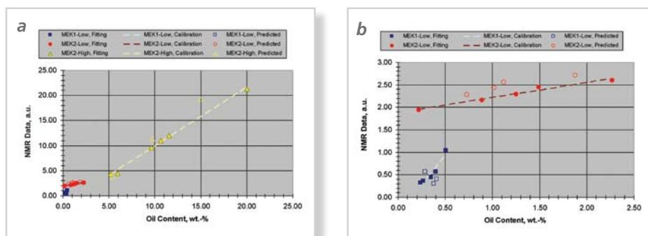
**Figure 1:** Graphs showing calibration data for (a) all, and (b) low oil content, wax samples. Solid symbols represent data points accounted in calibrations and used for fitting; open symbols correspond to data points excluded from fitting to improve standard deviations and correlation coefficients of the calibration procedure; dashed lines are the calibration curves.
