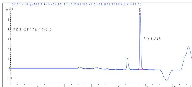
FIG. 2 and 3 When the OligoBead was used, no primer-dimer was observed even at 10 copies (left HPLC trace). Remaining primers were seen at 6.4 min and amplified product at 9.4 min. A Right HPLC trace shows the amplification of 100 copies with an oligobead of the same lot. Lower primer peaks and higher target peaks are observed.
