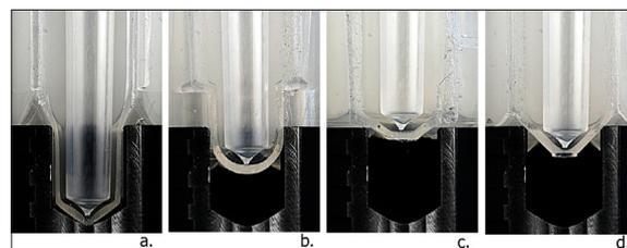
Figure 1. The sectional view of the Microtiter Deep Well 96 plate (1.a) and deep well 96 plates of other manufacturers (1.b, c and d) and the KingFisher Flex 96 deep well heating block
