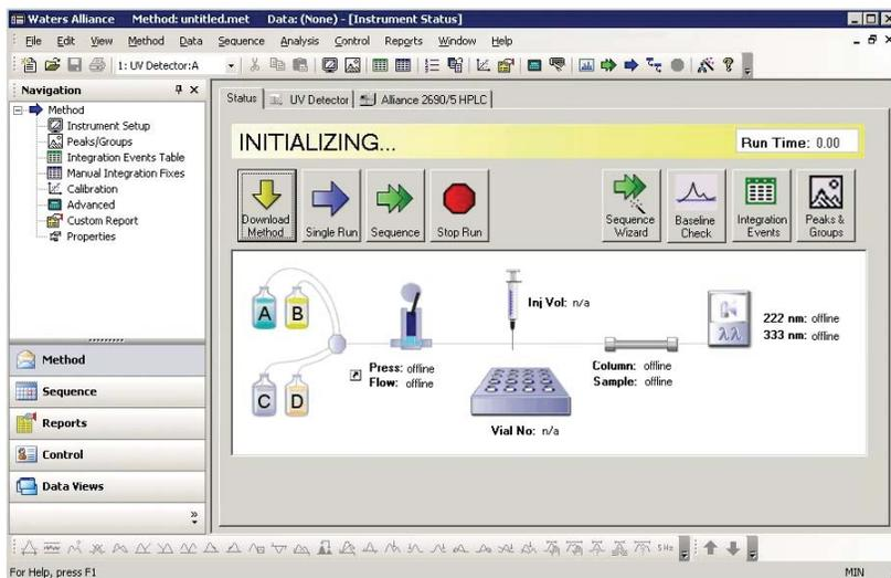
Figure 4: Typical instrument control screen from an OpenLAB web client. Real time status display of the instrument's condition can be instantaneously obtained. The above screen is taken from an OpenLAB web client in the act of initializing instrument control parameters to a supported Waters Alliance HPLC. OpenLAB instrument control of the Waters Alliance pump, autosampler, and detector is provided.
