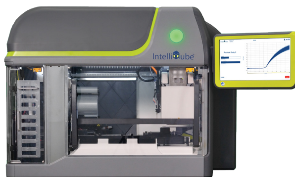
Figure 1: The IntelliQube is a fully integrated liquid handling and real-time quantitative PCR instrument optimized for use with miniaturized reactions in 768-well Array Tape.
