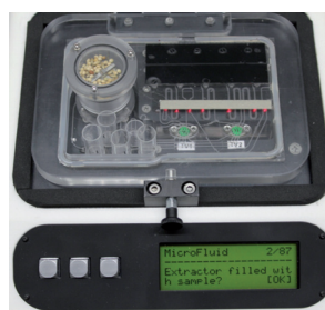
Fig. 1: Disposable polymer chip with attached extraction unit inserted into the fully automated device incl. actuation and detection modules.
