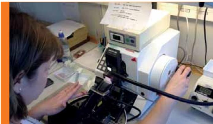
TMA sectioning within the SciLifeLab Uppsala tissue profiling facility, using a Thermo Scientific HM355S microtome with peltier-cooled attachment (Thermo Scientific Cool Cut) and Thermo Scientific Section Transfer System.
