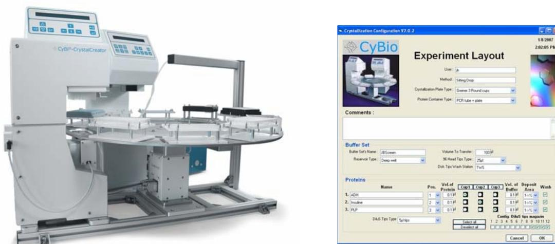
Figure 1: CyBi®-CrystalCreator, consisting of a 96-channel and an 8-channel automated pipettor mounted onto a 10-position deck equipped with an active tip wash station (left). The intuitive Graphical User Interface, which enables easy access to predefined programs (right).
