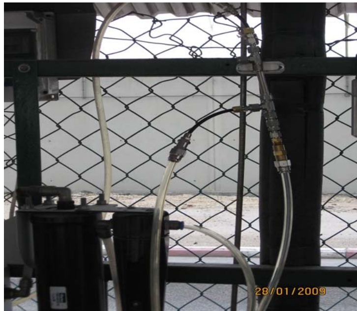
Fig.7. NTNU Nano-Membrane Module Installed in the Test Rig.
