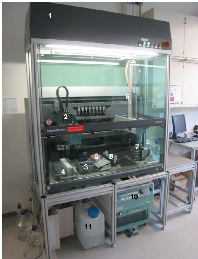
Figure 1 System overview; 1. Biosafety cabinet, 2. LiHa, 3. Te-Shake™ with chamber slides, 4. Reagent troughs and LiHa wash station, 5. Sterile system liquid, 6. RoMa, 7. Flask Flipper, 8. Te-Shake with tubes, 9. Tilting rack, 10. Centrifuge, 11. Liquid waste. Not all components are required for this application.
