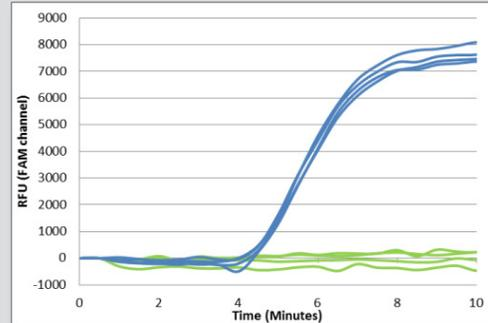
Figure 2. Exported results from AmpliFire (Time vs. RFU) using a crude *Salmonella* preparation method from boot swabs.
