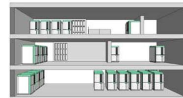
Large arrays of comPOUND stores can be distributed where it is convenient for the user. Sample tubes are then transported using pneumatic technology to the point of use.
