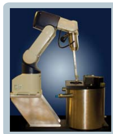
Figure 3. BRUNO II robotic sample handler
