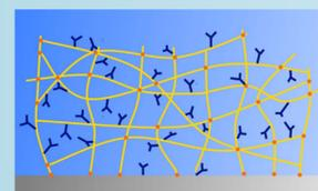
Schematic illustration of a spot containing antibodies immobilized in polymer network
