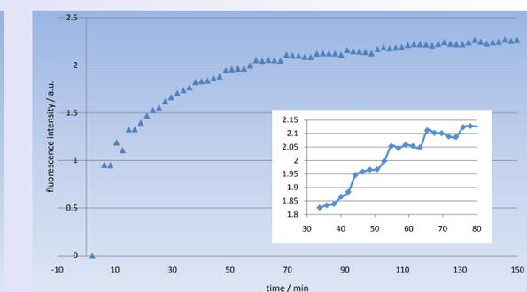
Dependence of stop-flow actuation on the fluorescence signal. Concentration of Cy5-labeled human IgG in solution: 8 nM. Duration static phase: 5 min, dynamic phase: 1 min
