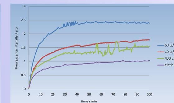
Dependence of the flow rate on the fluorescence signal. Concentration of Cy5-labeled human IgG in solution: 8 nM
