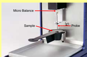
Figure 2. Image of a typical manual tensiometer used for conducting surface tension measurements
