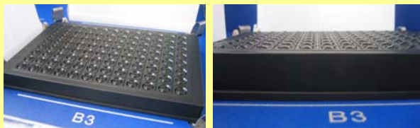
Figure 4. Uniform sample preparation for high throughput surface tension measurement.
