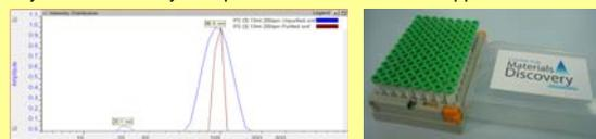
Figure 6. Particle sizing via DLS (left) shows particle distributions of a latex sample before (blue) and after (red) ten purification washings. Also the removal of small impurities can clearly be observed. The final library of multiple replicates of each latex sample is stored in robotically compatible 2D bar-coded vials and exported for application screening.
