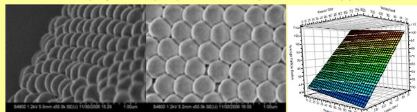
Figure 7. FE-SEM is used to image the aligned latex product to show the reproducibility in particle size and shape (left). Response surface modelling (RSM) is also used to illustrate the effects of mixing speed and reactor volume on latex particles size (right).
