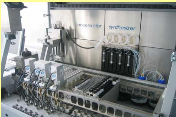
Figure 1. Chemspeed<sup>2</sup> SLT 106 set up with 13ml, 27ml and 75ml reactors to conduct HT latex synthesis investigations via experimental design.
