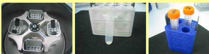
Figure 5. The latexes are centrifuged in batches of 48 samples for 20 minutes (left) and the pelleted samples returned to the liquid handler (centre). The process is also fully scalable for samples from larger reactor sizes up to 100ml (right).
