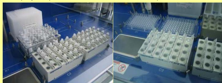
Figure 4. The samples are delivered from the Chemspeed automated synthesis platforms and placed directly onto the deck of an Eppendorf epMotion 5075LH liquid handling platform where the centrifuged samples are rapidly prepared and processed.
