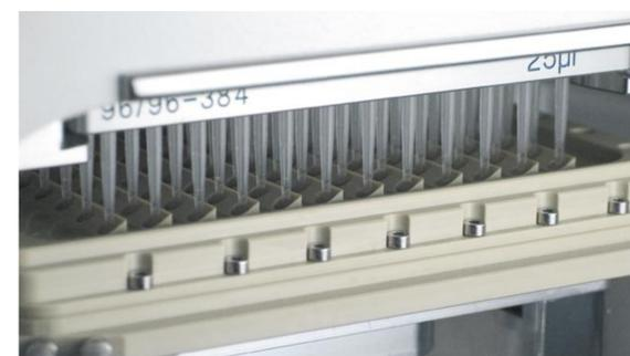
**Figure 2:** The active tip wash station utilizes independent clean water chimneys, in this case the 96 tip version, with its separated lower waste reservoir for disposal of liquids ensuring a constant flow of clean untainted wash solutions. It has a source channel and waste flutings for an inflow exchange of solutions for the cleaning of tips. This is driven by two peristaltic pumps.
