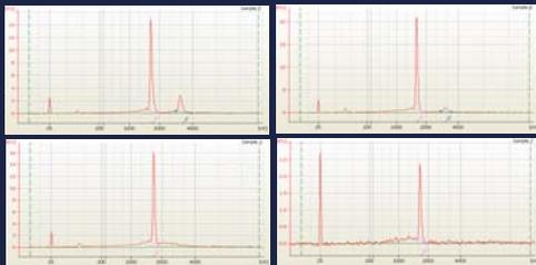
Figure 2. RNA integrity assessment by bioanalyser analysis. Electropherograms of different lysing methods are shown, a. mixing with glass balls, b. mixing with steel balls, c. sonication, d. chemical lysis
