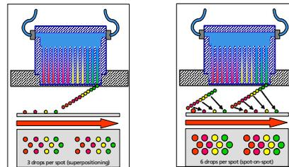
Figure 3: Illustration of superpositioning and Spot-on-Spot on-the-fly printing.
