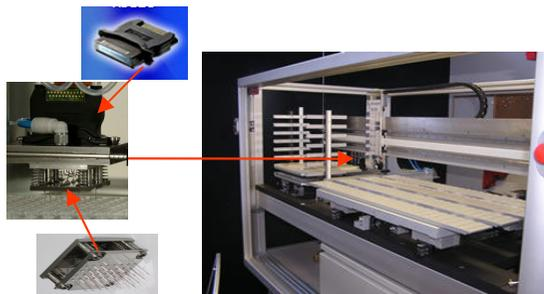
Figures 2a, 2b, 2c: & 2d: Arrayjet printer, close ups of the printhead and Jetspyder™ extracting samples from 384 well plate, and close ups of print head and 32 sample Jetspyder™.
