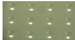
Figure 4: Multiple spotting of Cy3, 1nl spots on GAPS II viewed wet under the microscope.
