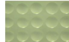
Figure 8: 1nl spots of IgG in Aj buffer printed onto PATH at 300um pitch.
