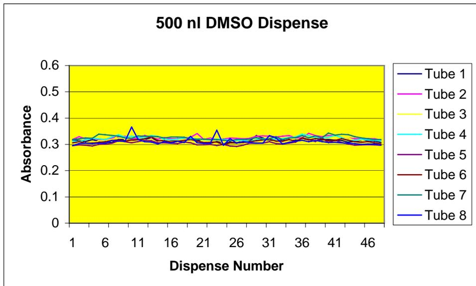
**Figure 6. Valve-to-Valve Uniformity.** DMSO containing a dye tracer (500 nl) was dispensed into a 384-well plate. After dispensing, 100  $\mu$ l of water was added and the absorbance at 630 nm of each well was measured using a Synergy™ HT Multi-Detection Reader. The data was then exported to Microsoft Excel and each valve tube's dispense was plotted separately.
