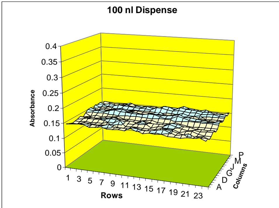
**Figure 5. Uniformity of Dispense.** The NanoQuot™ Microplate Dispenser was used to dispense 100 nl of aqueous dye solution into 384-well microplates. After the addition of dye solution, 100  $\mu$ l of diluent was added and the absorbance for each well determined. Data for the entire plate was plotted using Microsoft Excel.
