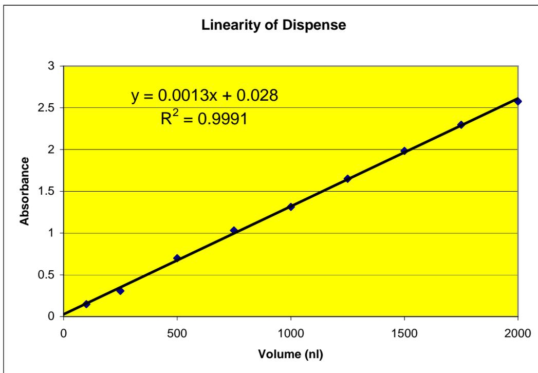
**Figure 4. Linearity of Dispense.** Different volumes of aqueous dye solutions were dispensed into wells of a 384-well microplate and the absorbance of each well was measured. The data for each plate was then exported to Microsoft Excel and plotted. Each data point represents the mean of 384 determinations.
