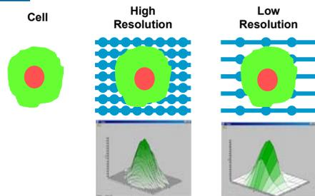
Scanning resolution can be defined in both X and Y directions. Construction of 3D fluorescence intensity profiles permits the calculation of fluorescence and morphological parameters for each object identified.
