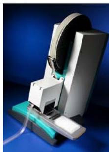
mosquito is a low volume liquid handling instrument combining a low-cost disposable tip system with a positive displacement pipette to ensure zero cross-contamination.
